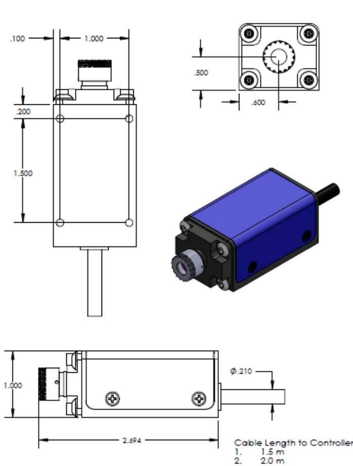
**NOTE:** H-Type Tethered Head comes standard with beam expander for spot size  $\sim 1.5$  mm and divergence  $< 1$  mrad
